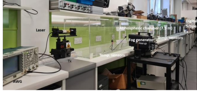
Fig. 2.6. Representative photograph of the atmospheric chamber under use in this test.
